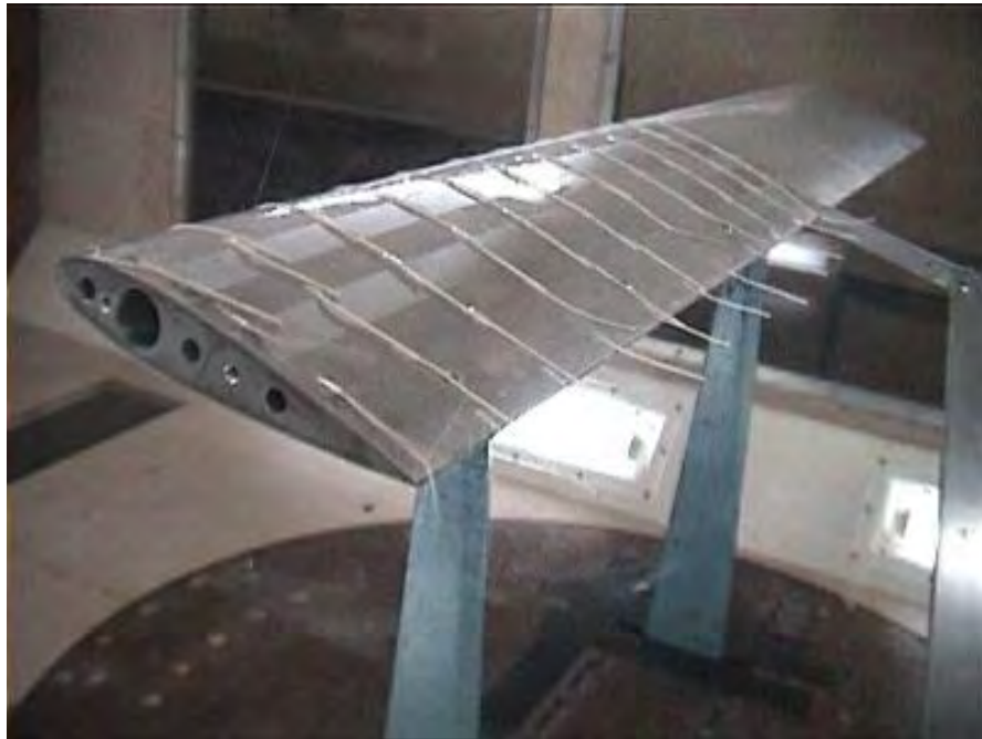
Figure 9.10: Test blade mounted in the wind tunnel
