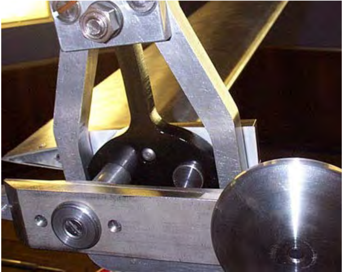
Figure 9.8: The ‘Type A’ elastomeric blade mounting component on the turbine rig.
