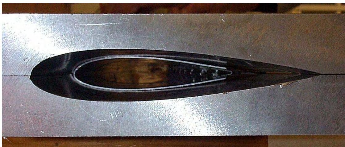
(b) Blade skin in mould used for clamping while the glue set
