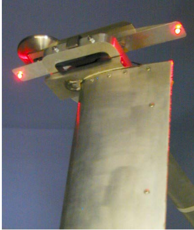
Figure 9.13: The target LEDs mounted on one of the blades.
