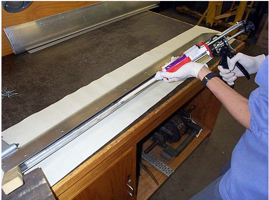
(a) Application of glue to blade trailing edge
