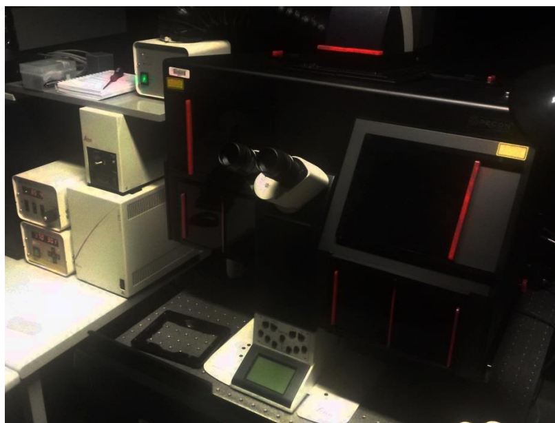
Figure 6.29: Leica DMi8 live cell imaging microscope equipped with dedicated incubator and CO 2 and temperature control.
