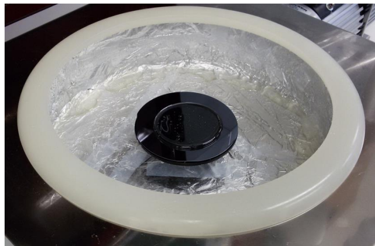
Fig. F.4: Dispensing the photoresist on silicon wafer. The bubbles generate should be avoided.
