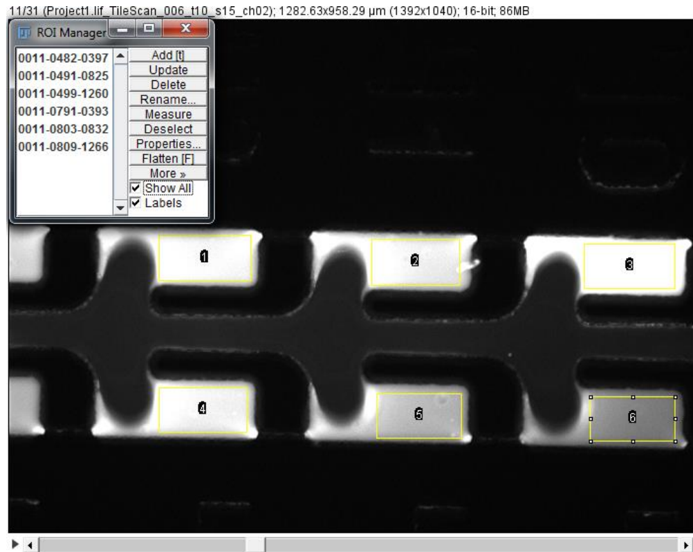
Figure 6.32: Image showing the use of ImageJ for defining ROI and measuring the fluorescent intensity.
